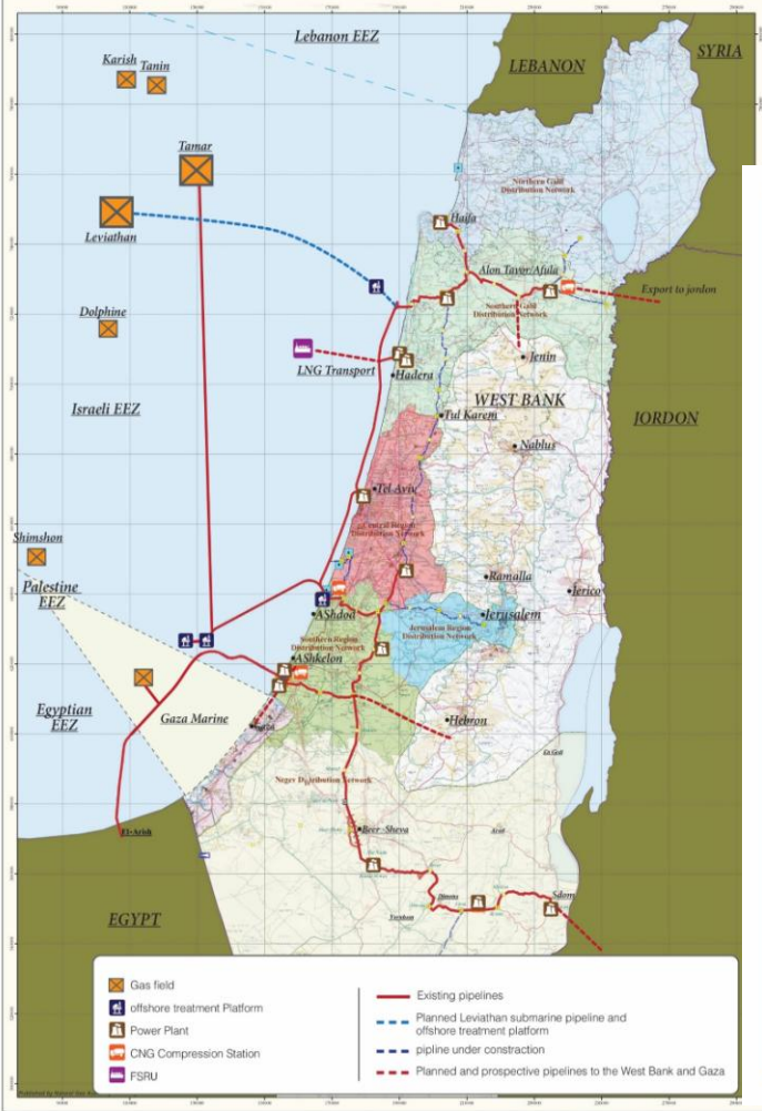
Israel and Palestine Authority's Gas Fields, High Pressure Natural Gas Transportation Network and Region of Low Pressure Distribution Companies
